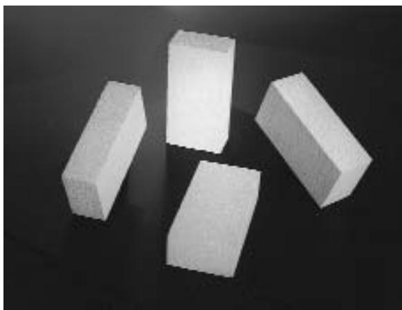
The SR-90, SR-99, and SR-99 firebricks are premium high alumina firebricks that are capable of handling very difficult applications. These premium bricks are very dense and have excellent load bearing strength at temperatures above 3000°F (1649°C) and they provide excellent thermal shock resistance. The extremely low silica content of both products make them ideal for hydrogen atmospheres.
